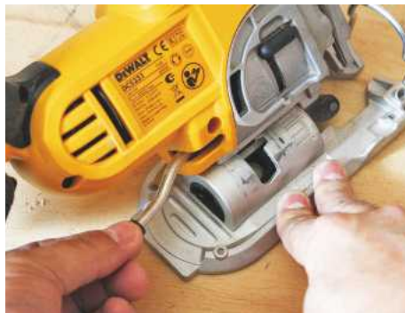
▲ The base can be tilted up to 45° by releasing this locking lever
